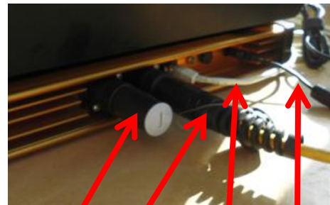
data end plug towards HPU power towards laptop
