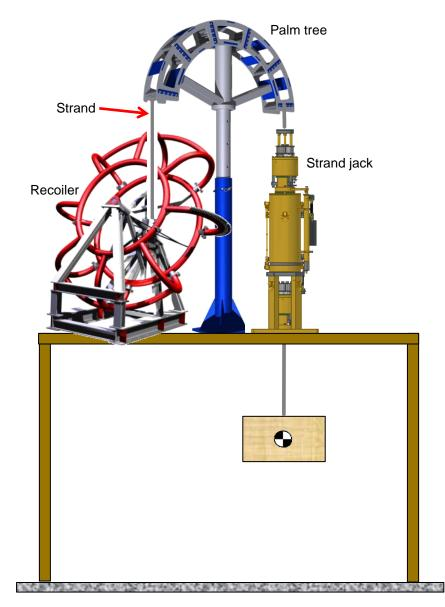
The recoiler rotates by the pulling and pushing forces of the strands.
