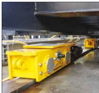
▼ ETR-Series electric trolley undergoing factory acceptance testing prior to shipment.
